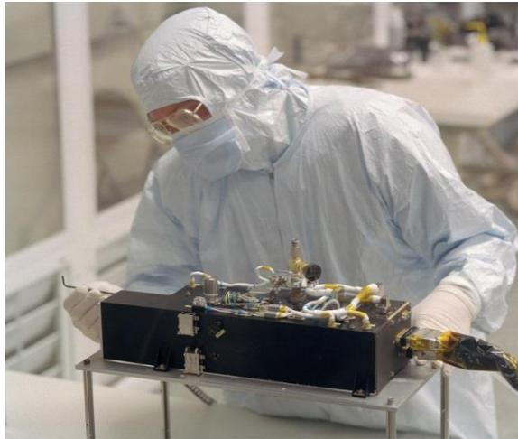
ALICE is imaging spectrograph in the  $\lambda\lambda 70\text{--}205\text{ nm}$ ,  $\Delta\lambda 0.8\text{--}1.2\text{ nm}$ . The slit,  $5.5^\circ$  long, with a width of  $0.05^\circ\text{--}0.10^\circ$ . Alice employs an off-axis telescope feeding a 0.15-m normal incidence Rowland circle spectro-graph with a concave holographic reflection grating. MCP detector utilizes solar-blind opaque photo-cathodes (KBr and CsI).
