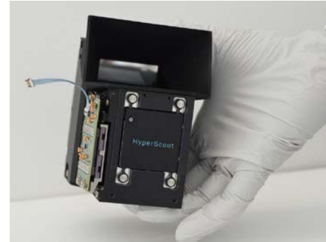
HyperScout. Hyperspectral imager (around 2 Kg and 10 W). Image source ESA.
