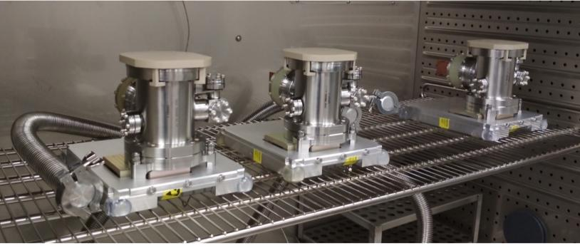
Fig. 2. EQM Enclosures at LPI climatic chamber before pump & bake procedure (Moscow, Russia).
