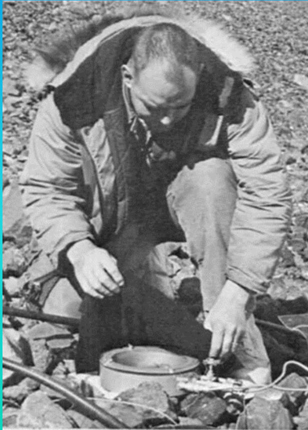
Ted Gannutz, USARP, Clark University, conducts lichen photosynthesis experiments with the aid of a respiration chamber.
